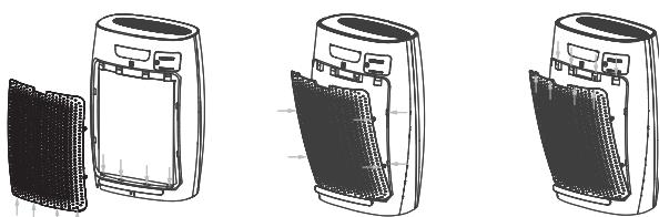
Insert the bottom buckle of the rear housing into the slot at the bottom of the body
