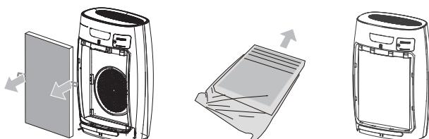
Hold the filter elements on both sides of the belt, remove the filter elements
